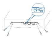
5. Connect the Exit light by sliding it into the base and engaging the terminal.
