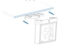
6. Then lock the Exit light in place by turning the clip to the right.
